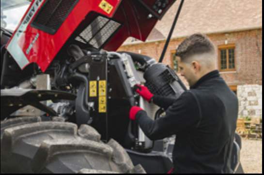
Cooling package is easily accessible to make cleaning faster and easier.
